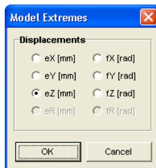
**Select the eZ displacement** component, and press **OK**. The location and value of the negative maximum displacement pops up in a window. Pressing **OK** closes it, and the positive maximum displacement window pops up. Press **OK** to close it too.
