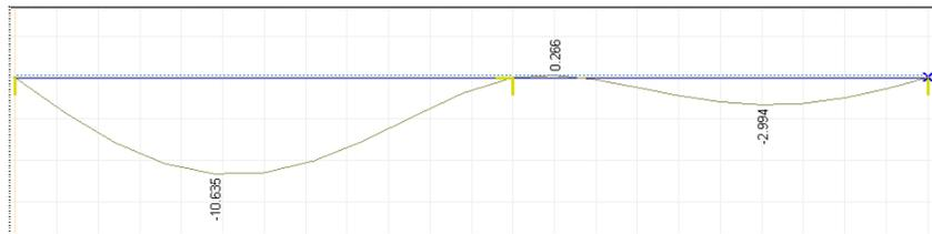
Check the displacement diagrams of various load cases whether they comply with the expected result. To do this, **click on the combo box** next to the Result Display Parameters Icon, and **select desired load** case. This time select the first load combination (Co. #1).
