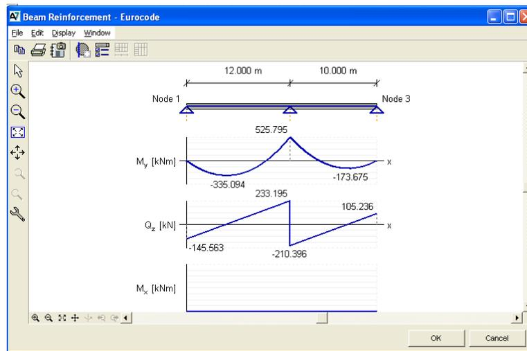
The topmost diagram is the static layout of the beam, below it is the  $M_y$  moment diagram and the  $Q_z$  shear force diagram.
