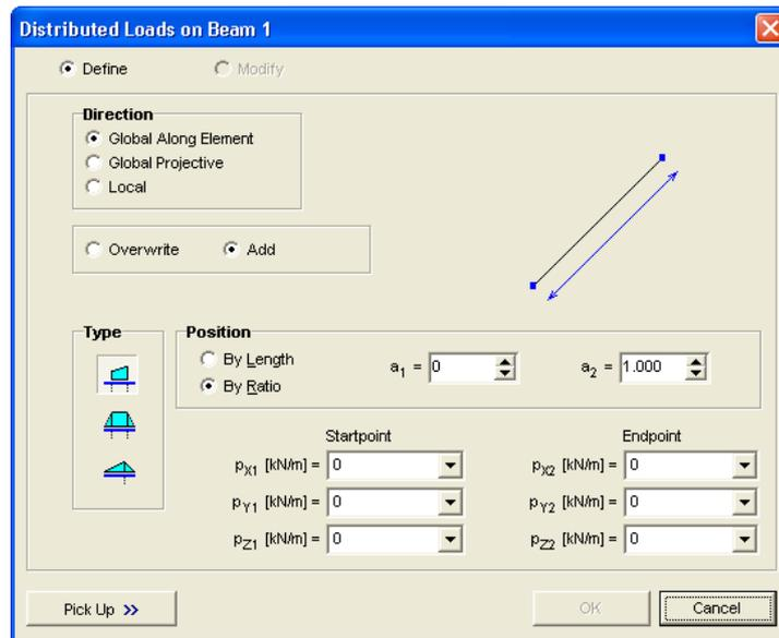
As the load intensity **type -17.5** in the p<sub>z1</sub>, p<sub>z2</sub> edit boxes, then press **Ok**.
