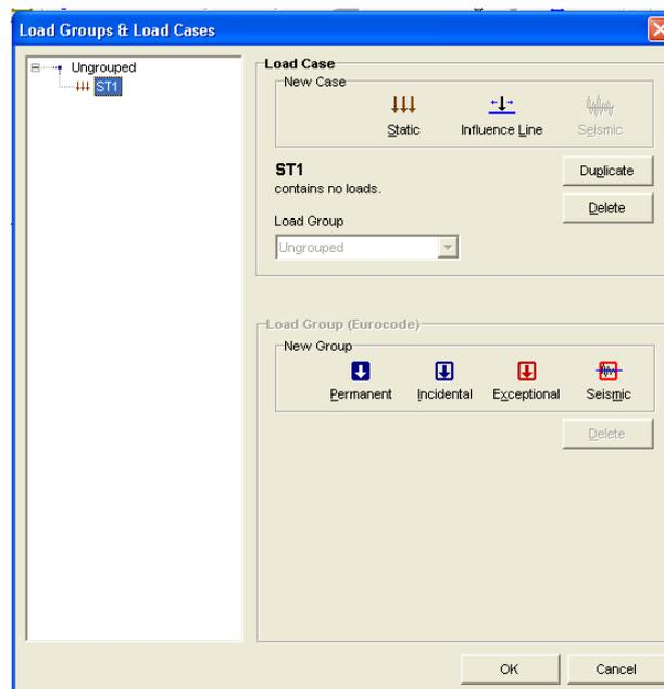
In the left tree view you can see the first load case, created automatically by the program. Its name is ST1. **Click on the ST1** to change the name of the load case, and **overwrite it with SELF-WEIGHT**. Click **OK** to return to the graphics area. The active load case will be SELF-WEIGHT. You can see it on the Info Window.
