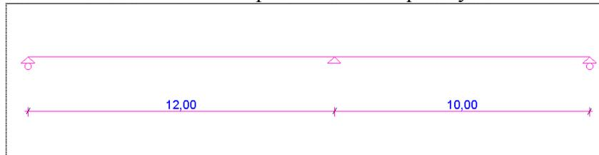
The analysis will be done according to the Eurocode. The cross-section of the beam is will be a 400mm x 600mm rectangle. The left beam is 12m in length and the right beam is 10m.
