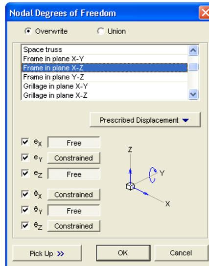
This setting selects the nodes of the beams only in translation in plane X-Z with the rotation around the Y-axis.
