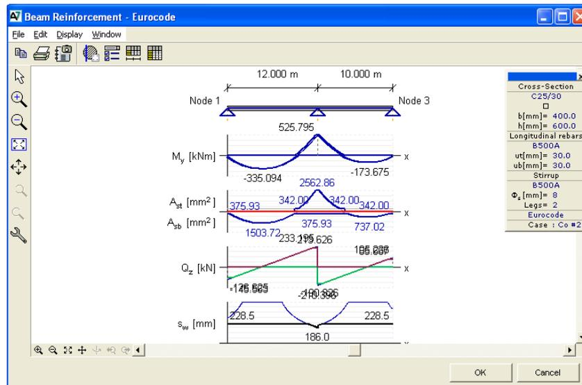
Note that alongside the original  $M_y$  moment diagram (thin line), the diagram shifted according to code (thick line) is also present. Below the  $M_y$  moment diagram is the  $A_s$  diagram, below the  $Q_z$  diagram is the  $s$  diagram.
