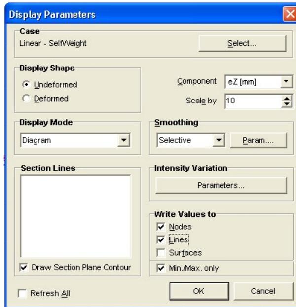
In the Case Selector combo box **select the SELF-WEIGHT** load case. If you leave the Undeformed radio button checked in the Display Shape panel, then the various results will be drawn on the undeformed shape of the structure. In the Component combo box **select ez** from displacements. **Set the Display Mode** to diagram. In the Write Values To Panel **check Nodes and Lines**. Close the dialog window with **Ok**. You should see the following picture:
