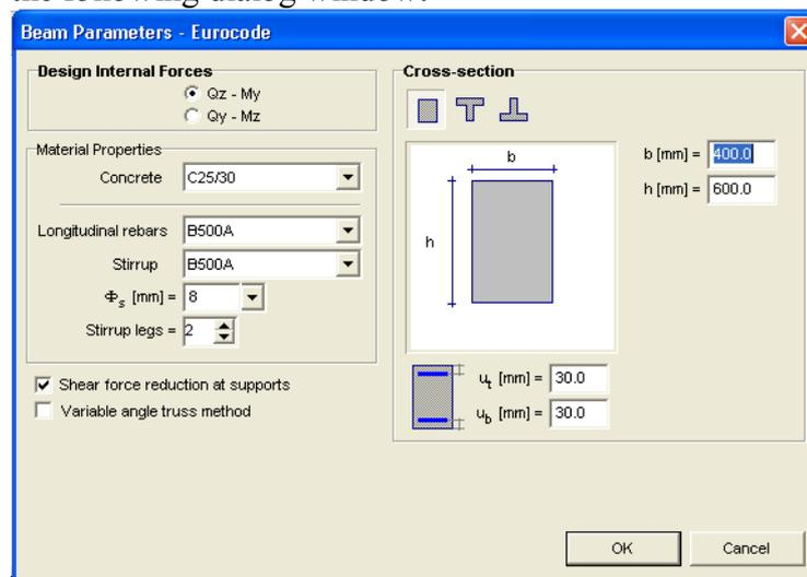
Set the **longitudinal rebar** and stirrup material property to B500A.
